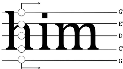
Figure 1. Adapted from Cooper (1950). The figure shows how the Optophone scanned a line of text. The scanning spots moved horizontally over a line of text. Where black print was encountered by a spot, a tone at the associated frequency was produced. The tones are labeled by their musical names on the right of the figure. Sometimes, as depicted just one tone was emitted. More commonly two or more tones generated a chord.
