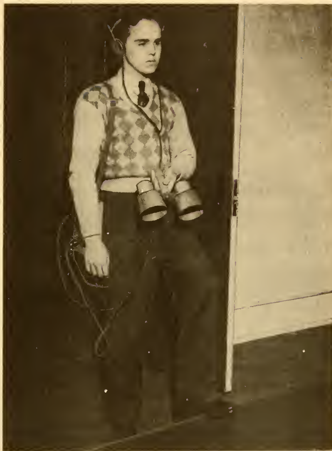
FIG. 2.6 SUBJECT CARRYING STROMBERG-CARLSON SUPERSONIC DEVICE, YA-3ST.
