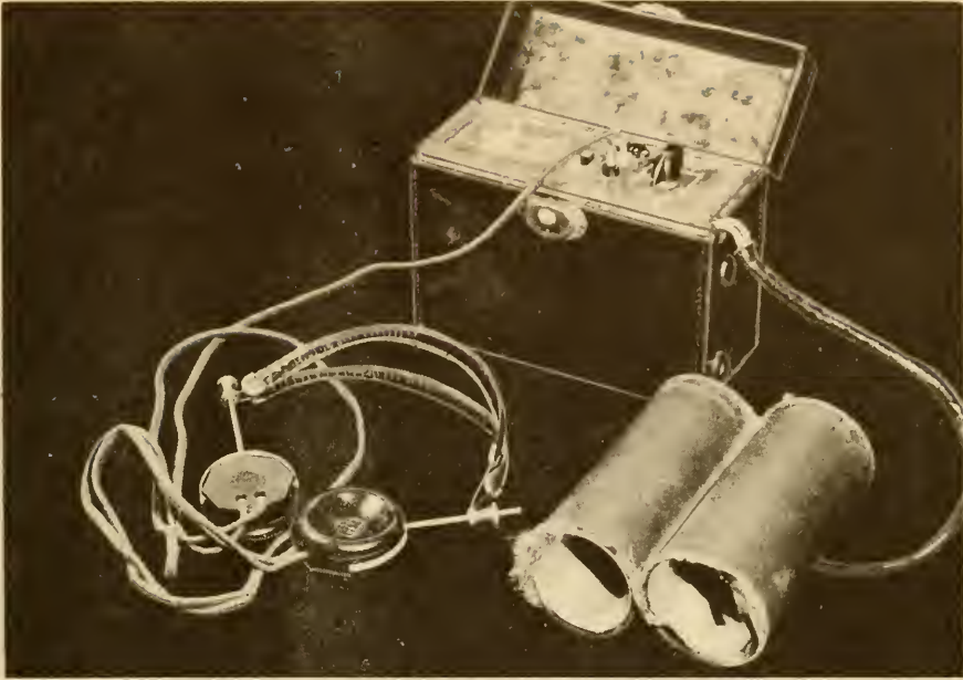
FIG. 2.25 BRUSH SUPERSONIC GUIDANCE DEVICE , YA-2BD.
