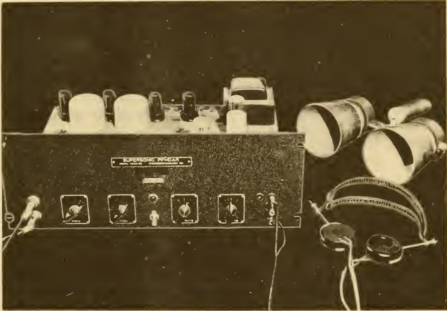
FIG. 2.29 STROMBERG - CARLSON SUPERSONIC GUIDANCE DEVICE, YA - 2ST.
